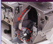
Simple looper threading
